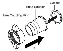
2. Thread the Hose Coupling Ring onto the Intake Port (a), and turn clockwise until fastened securely (b).
